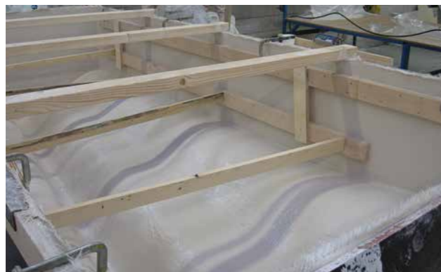
Element laminated and 36 mm plywood beams positioned to the sides
