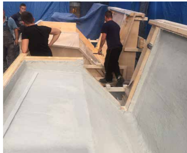
A1 element laminated in the mould
